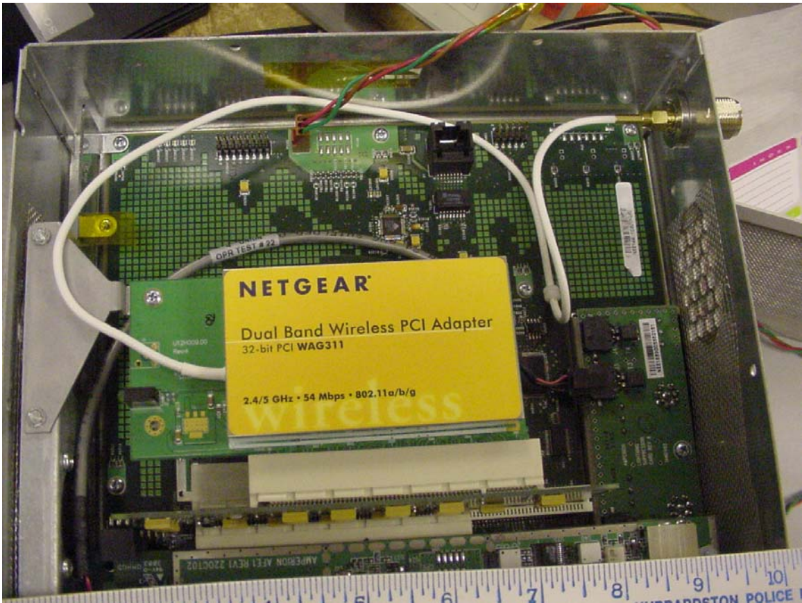
Interior of device enclosure with cover removed, close up of RF LAN card installation.
