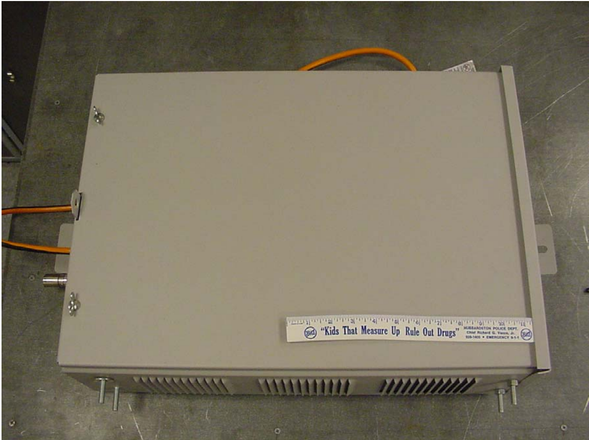
Exterior of NEMA Pole Mounted Enclosure (Front), showing cover installed
