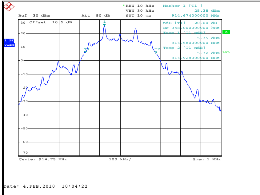
Figure 7.2.2-2: 20dB Bandwidth Plot – Mid Channel
