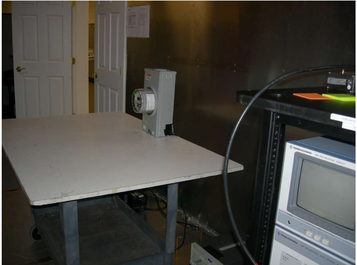
Figure 7: 2S Meter – AC Power Line Conducted Emissions
