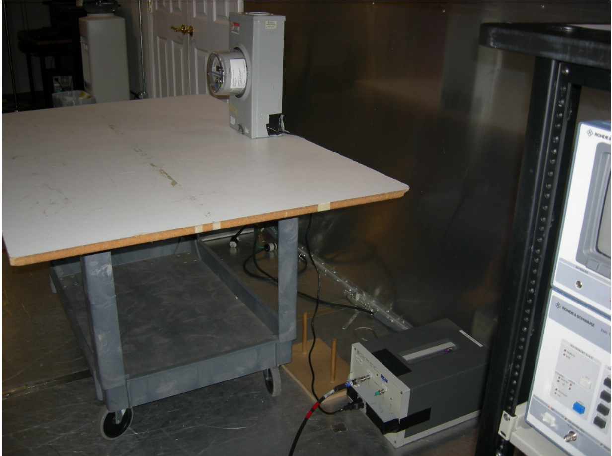
Figure 3: 1S Meter – AC Power Line Conducted Emissions
