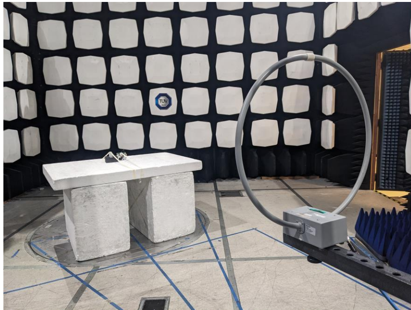
Figure1 – Test Set up - Radiated Emissions <30 MHz
