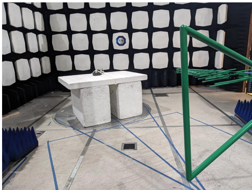
Figure2 – Test Set up - Radiated Emissions <1 GHz
