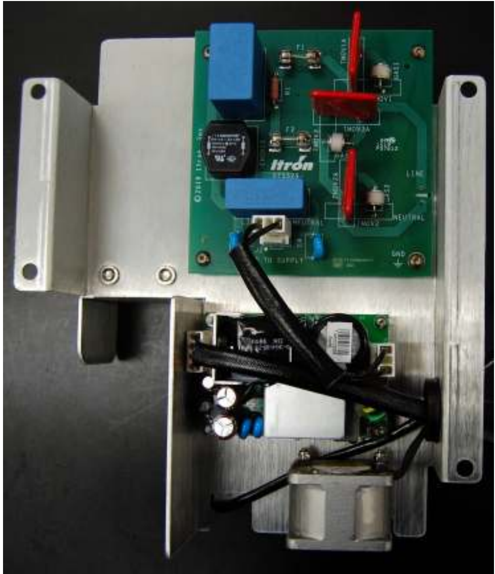
Power supply and protection board mounted in bracket
