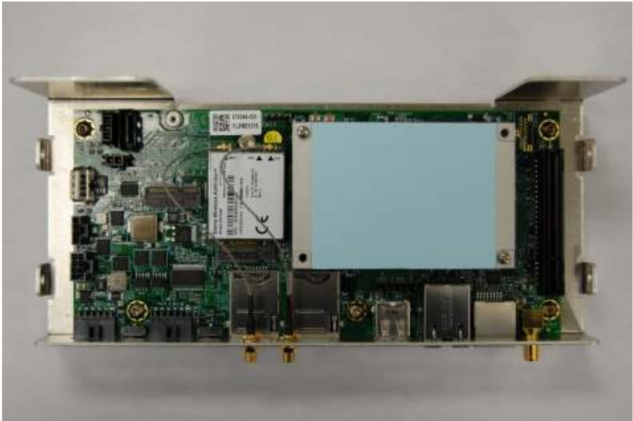
Adlink board mounted in bracket (modem installed)
