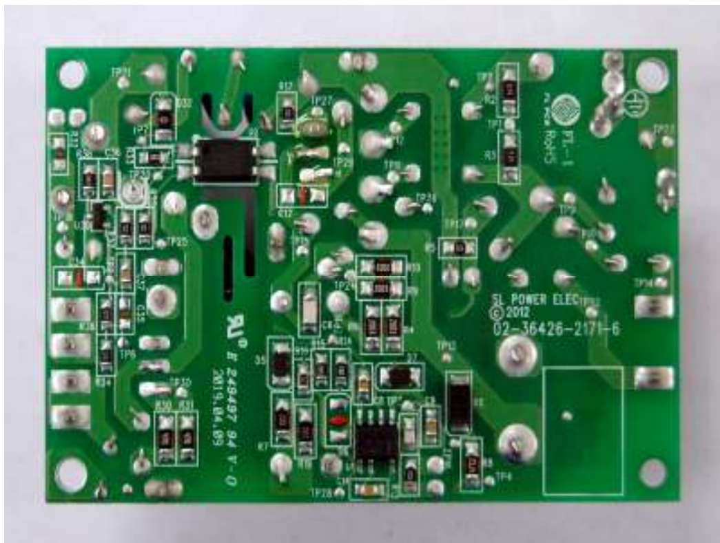
SL power supply, bottom
