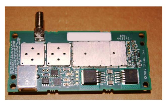
Figure 1 Itron ITR9002 module, FCC ID: SK9ITR9002
