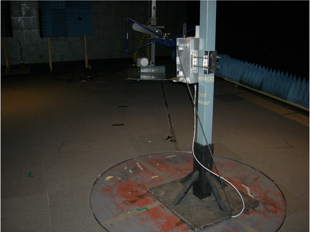
Figure 6: Radiated Inter-modulation Products (Itron Prism Cell Relay Host)
