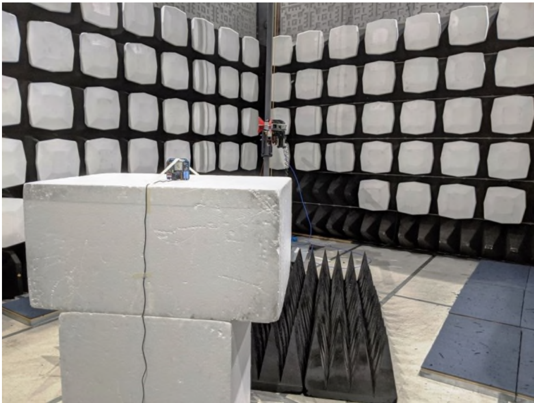
Figure 8: Test Setup – Radiated Emissions >1GHz
