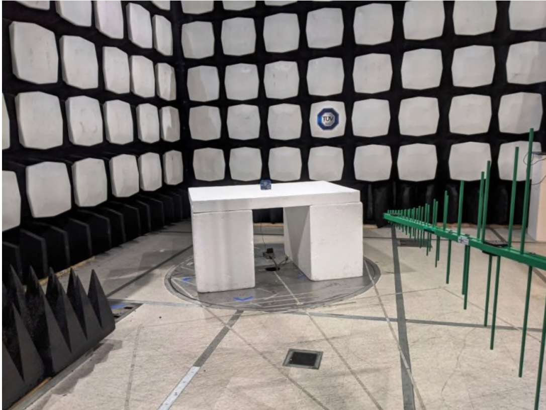
Figure 5: Test Setup – Radiated Emissions <1GHz
