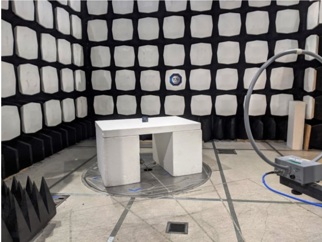
Figure 3: Test Setup – Radiated Emissions <30MHz
