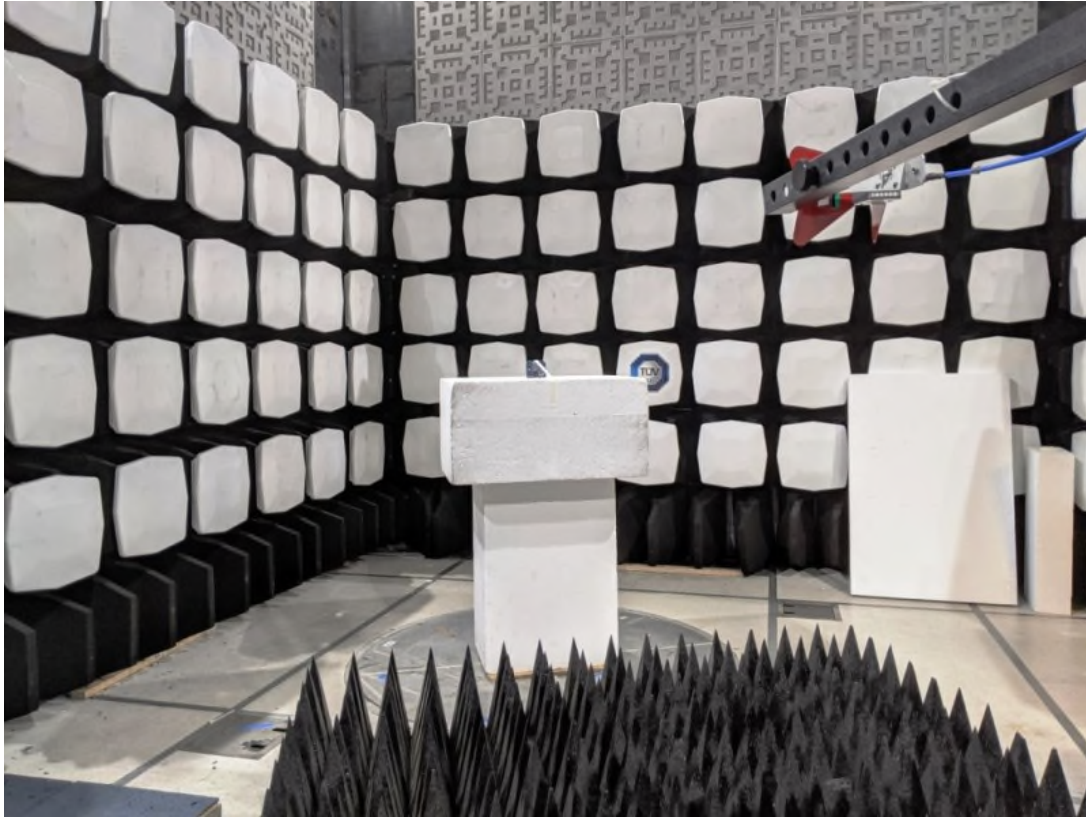
Figure 7: Test Setup – Radiated Emissions >1GHz
