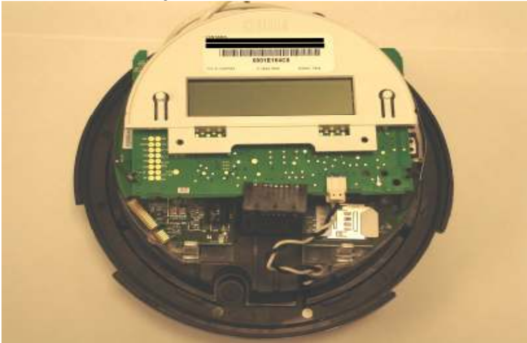
Meter Base with CAT2 and register boards installed
