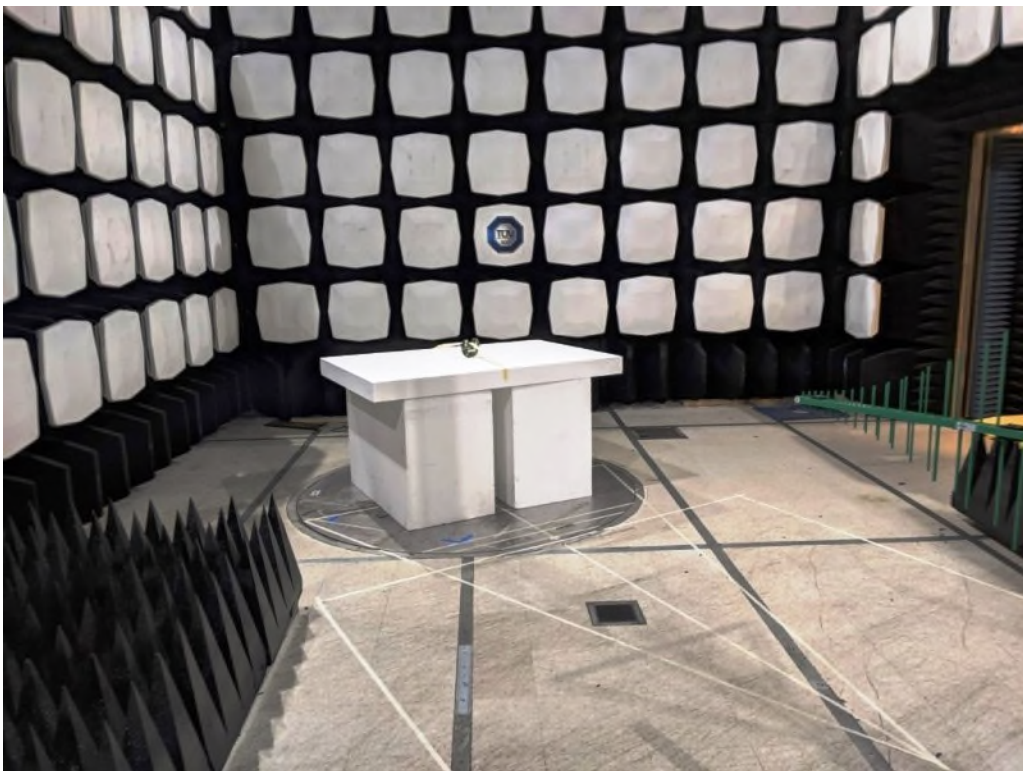
Figure 4: Equipment Under Test – Radiated Emissions <1GHz
