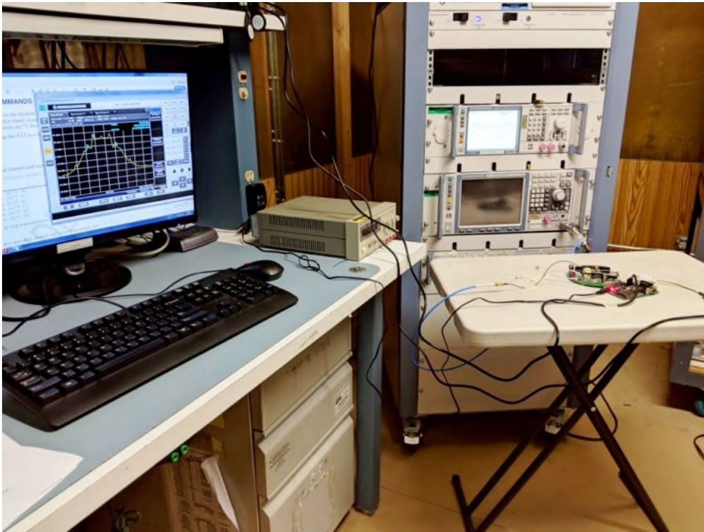
Figure 1: Equipment Under Test – Radiated Emissions – Antenna Port Conducted Measurements
