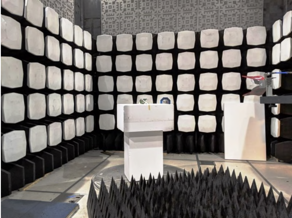
Figure 6: Equipment Under Test – Radiated Emissions >1GHz
