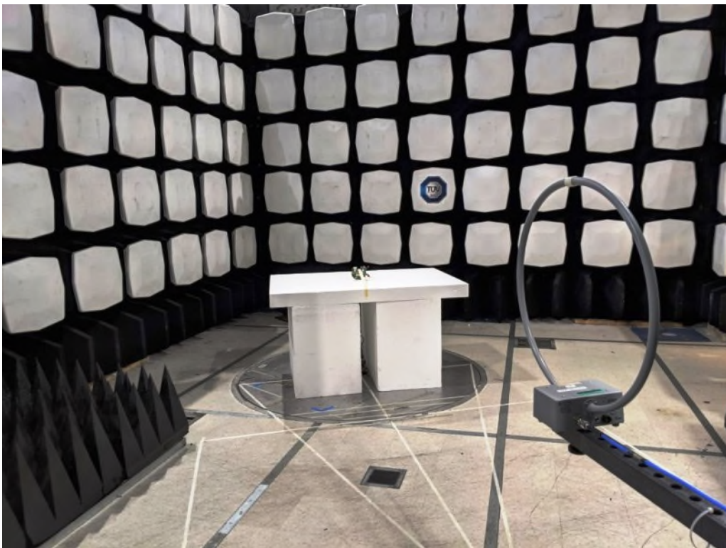
Figure 2: Equipment Under Test – Radiated Emissions <30MHz
