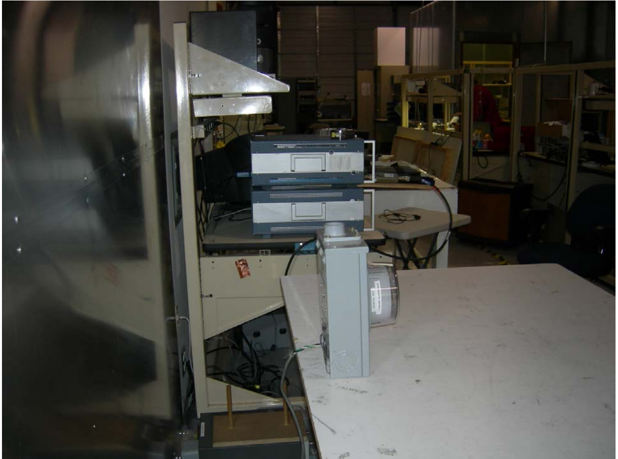
Figure 7: AC Power Line Conducted Emissions
