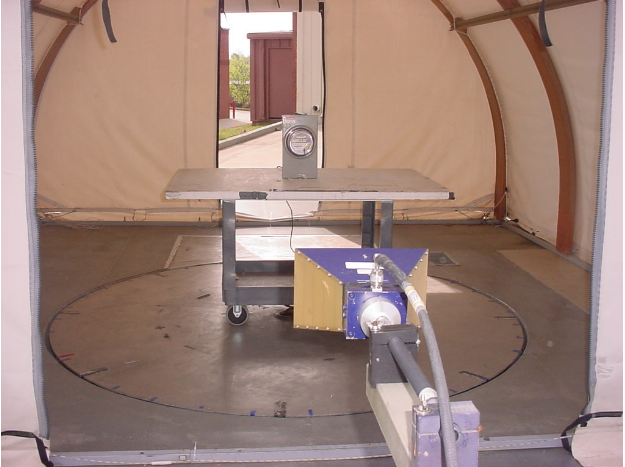
Figure 2: Radiated Emissions – Intentional
