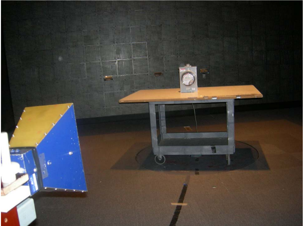
Figure 4: Radiated Emissions – Unintentional
