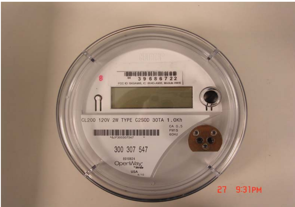
Figure 2: Itron AMI6 module installed in Itron meter form
