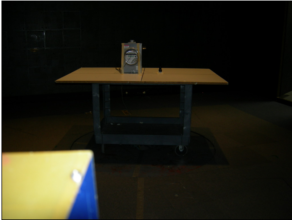
Figure 5: Radiated Emissions – Stub Antenna
