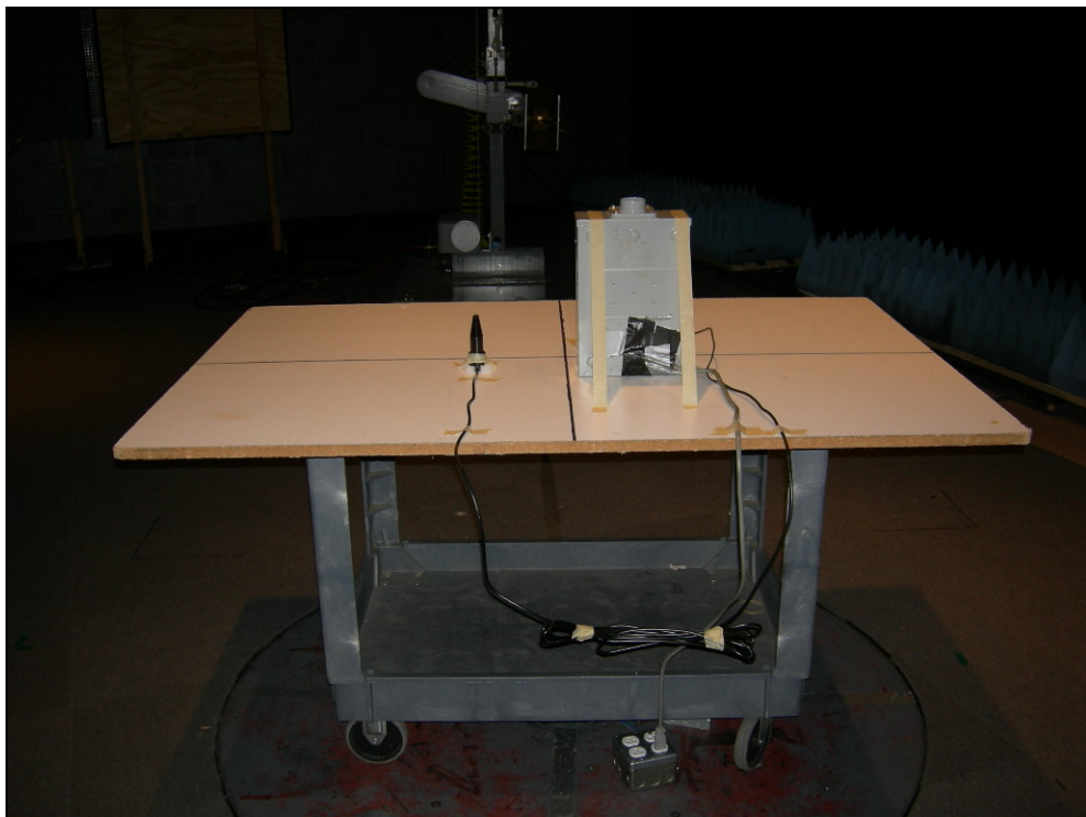
Figure 4: Radiated Emissions – Stub Antenna
