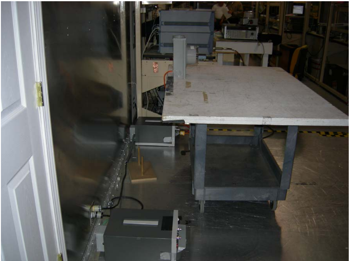
Figure 4: AC Power Line Conducted Emissions
