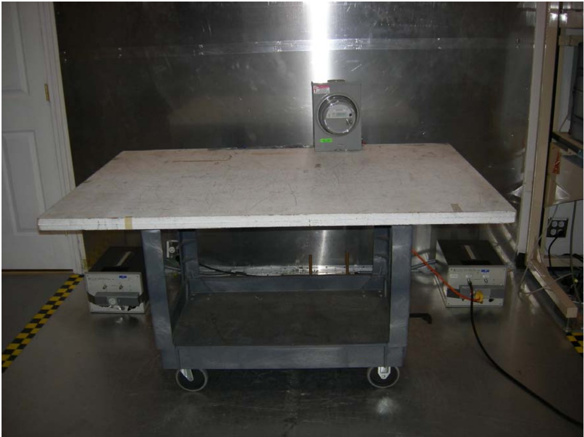
Figure 3: AC Power Line Conducted Emissions
