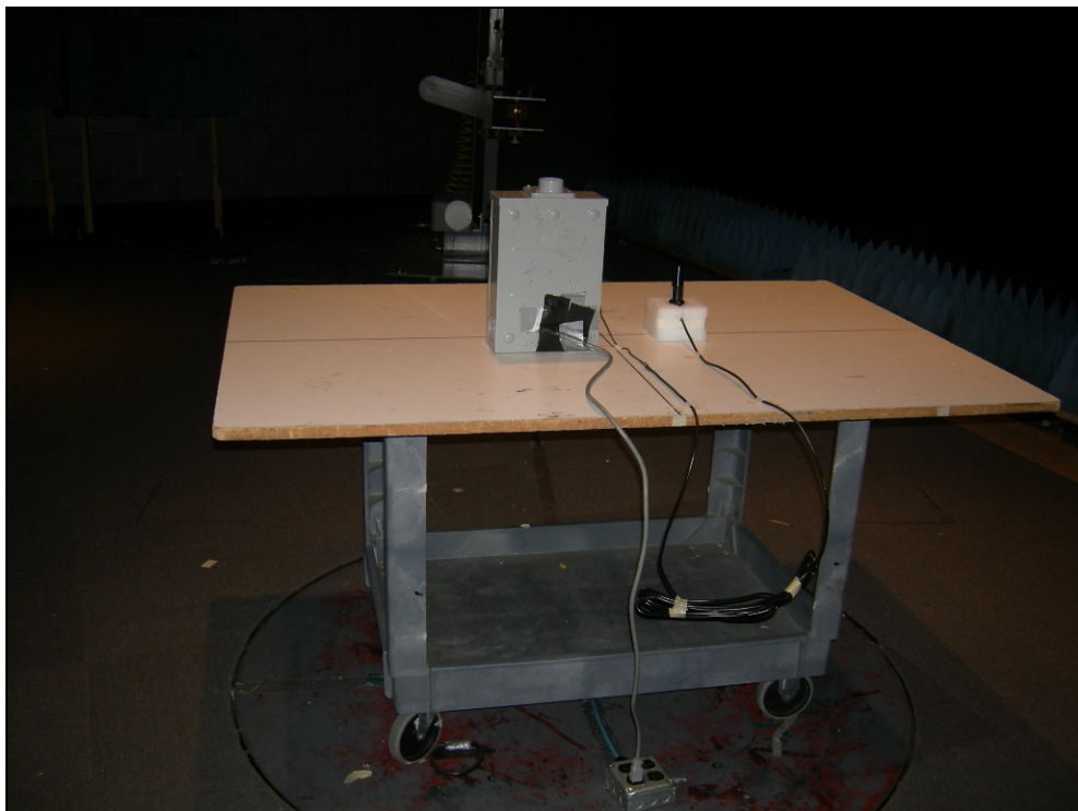
Figure 4: Radiated Emissions – Stub Antenna
