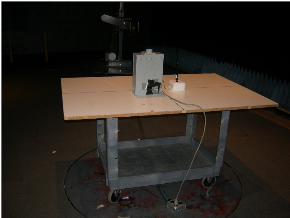
Figure 6: Radiated Emissions – Whip Antenna
