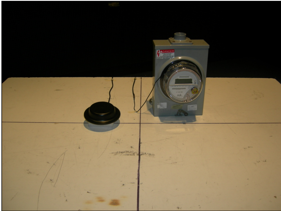
Figure 1: Radiated Emissions – Radome Antenna
