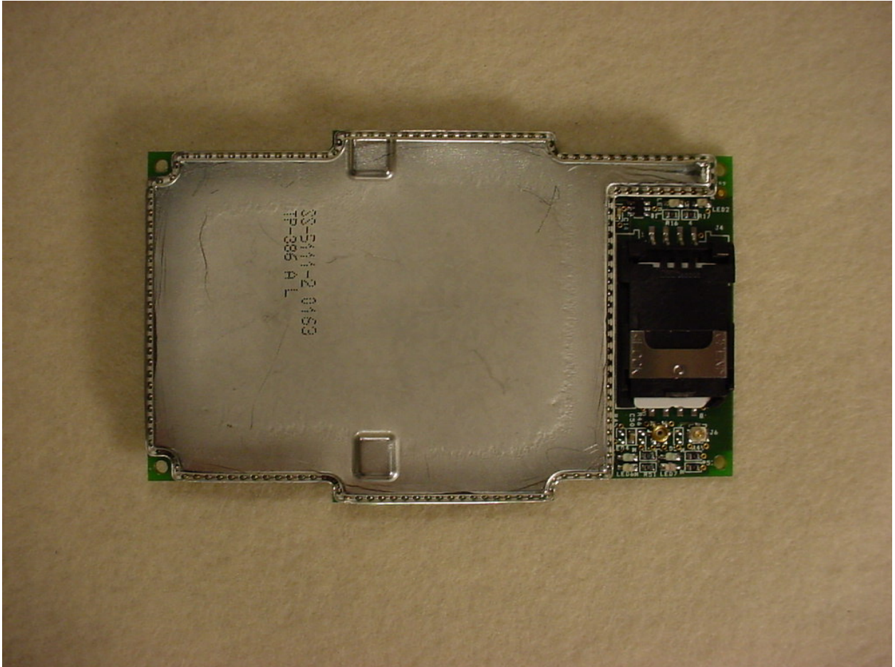
Figure 14: Internal – Mezzanine GPRS Board Front w/ Shields (GPRS & GPRS + Ethernet Sub Assemblies Only)
