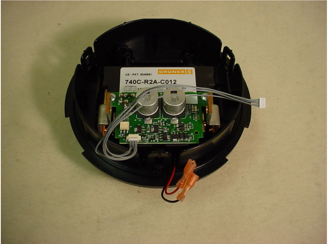
Figure 9: Internal – Disconnect Switch
