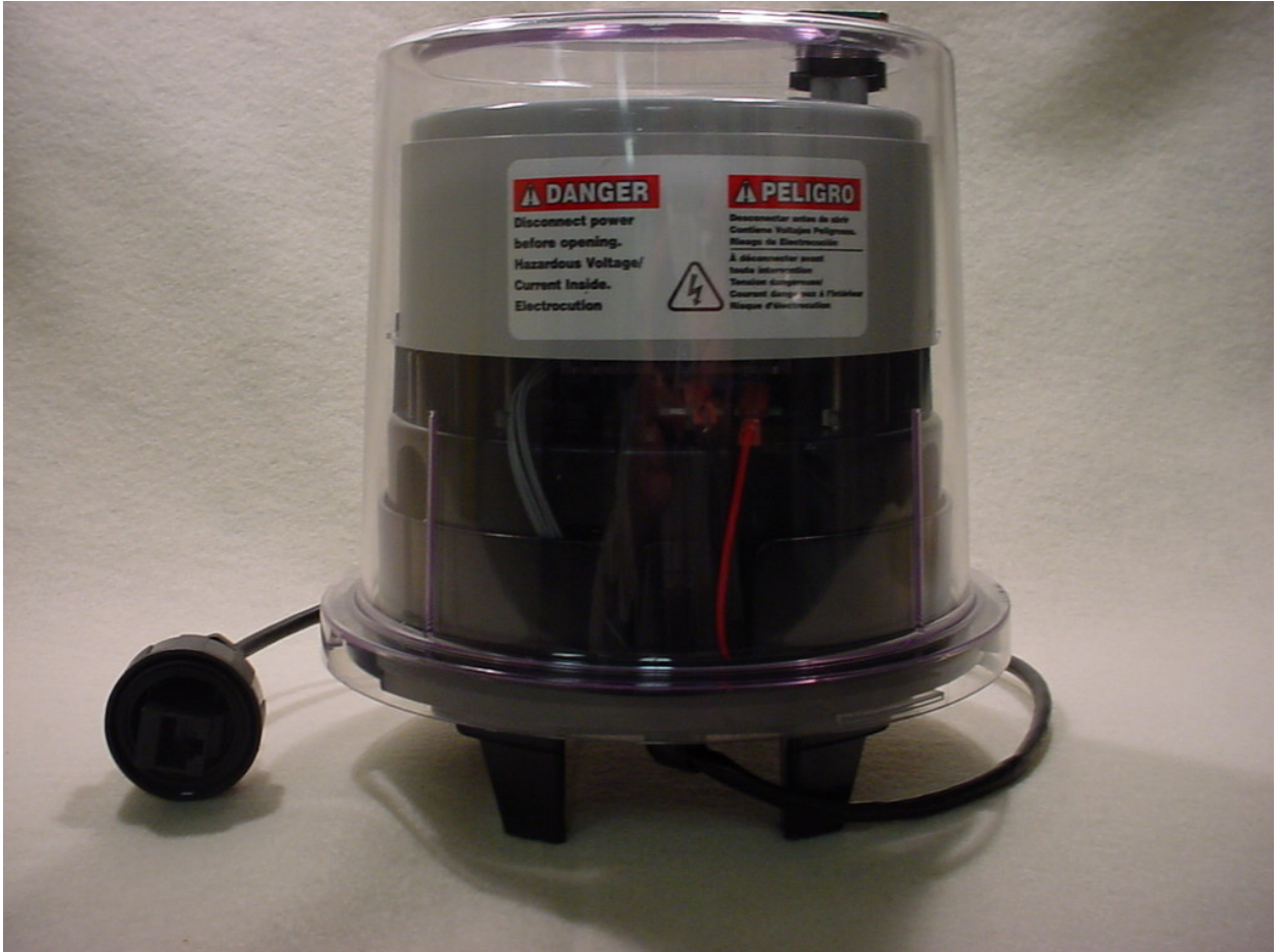
Figure 11: External – Side View (Ethernet Capable Sub Assembly)
