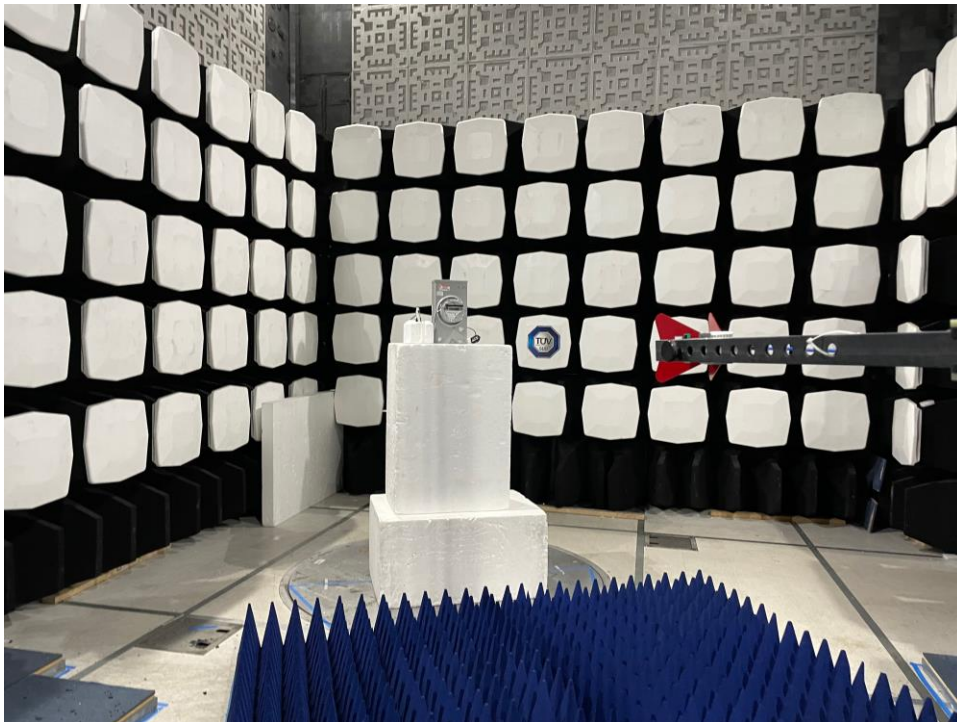
Figure 8: Equipment Under Test – Radiated Emissions >1GHz-Stub Antenna
