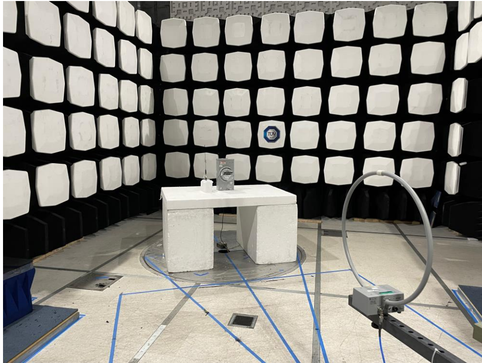
Figure 1: Equipment Under Test – Radiated Emissions <30MHz-Whip antenna
