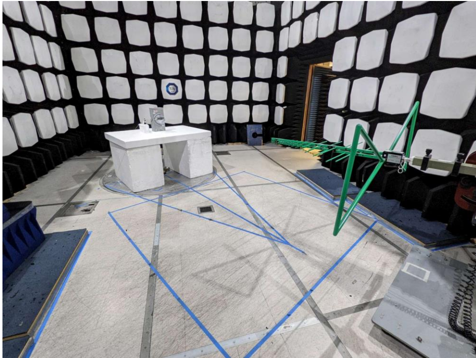
Figure 5: Equipment Under Test – Radiated Emissions <1GHz-Stub Antenna
