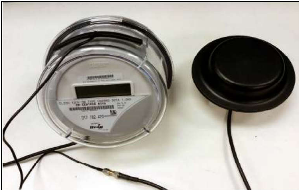
Figure 4: External Photo – Puck Antenna (Flex Coupler Attached to LP800 Antenna)
