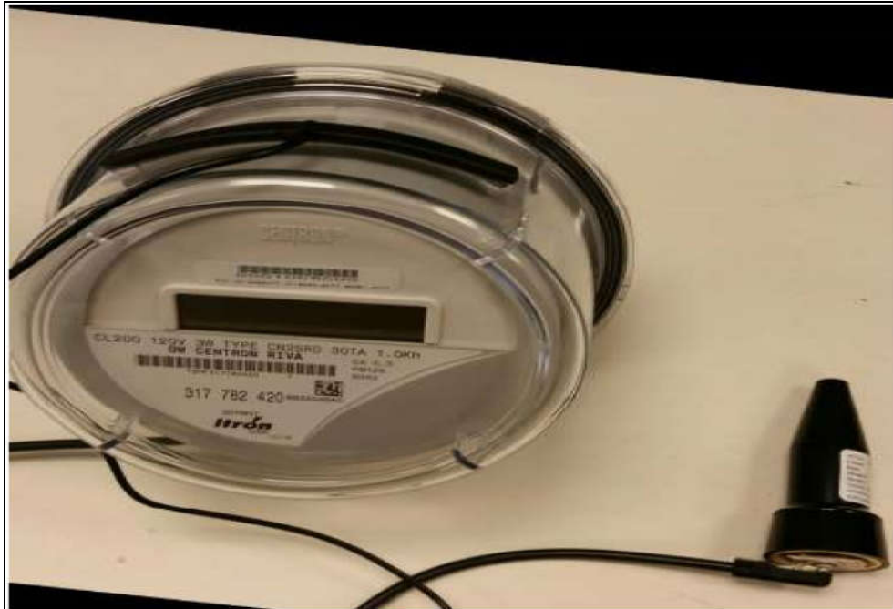
Figure 3: External Photo – Stubby Antenna (Flex Coupler Attached to A158192B Antenna)
