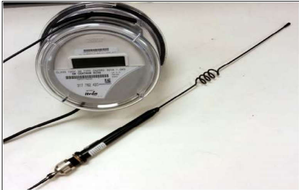
Figure 2: External Photo – Whip Antenna (Flex Coupler Attached for ASPG918 Antenna)
