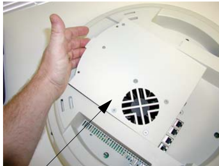
Access panel (with power supply and fan)
