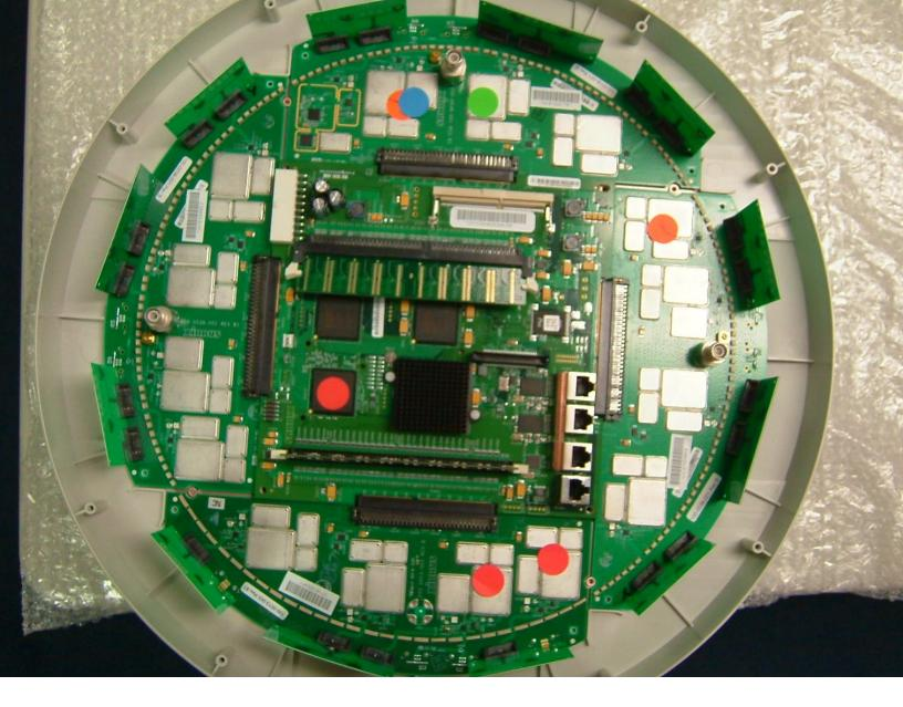
In the XS3700 the rf boards only have two transceivers per board. The board shown is for the XS3900 which has all four transceivers installed. A separate photograph of the rf board with only two transceivers has been provided."
