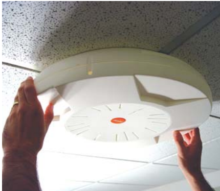
Figure 28. Attaching the Unit (XS-3900)
