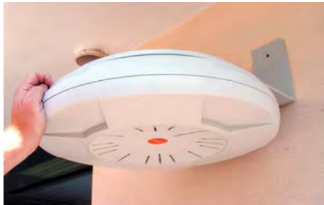
Figure 37. Mounting the Array on a Wall
