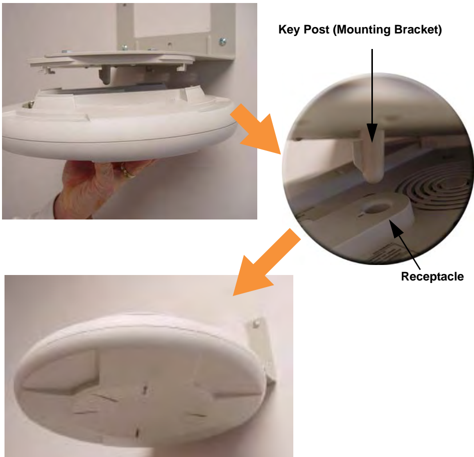
Figure 42. Mounting the Array on a Wall
