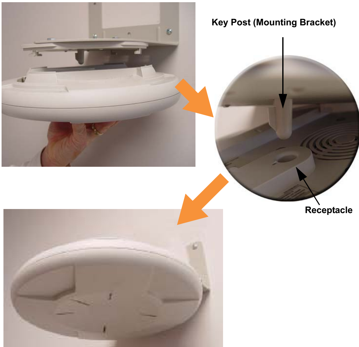
Figure 55. Mounting the Array on a Wall
