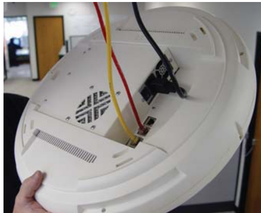
Figure 40. Connecting the Cables
