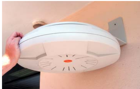
Figure 50. Mounting the Array on a Wall
