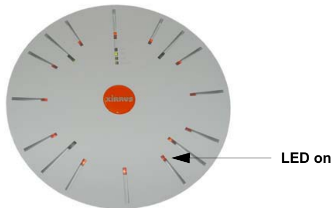
Figure 103. LEDs are Switched On
