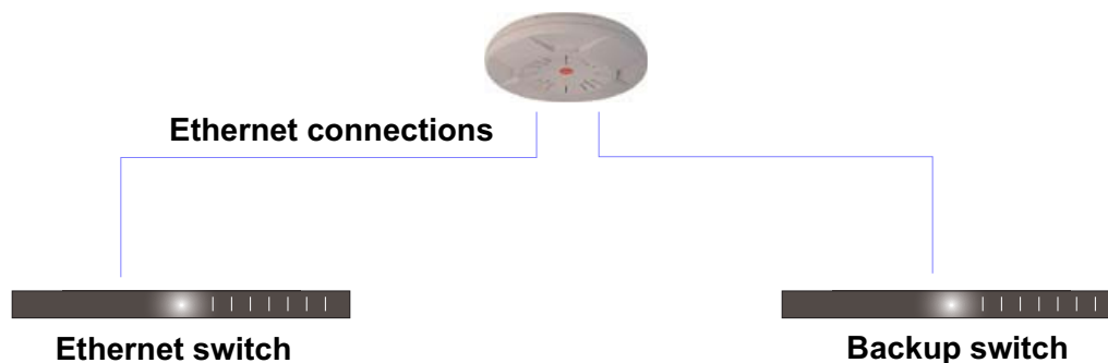
Figure 30. Switch Failover Protection
