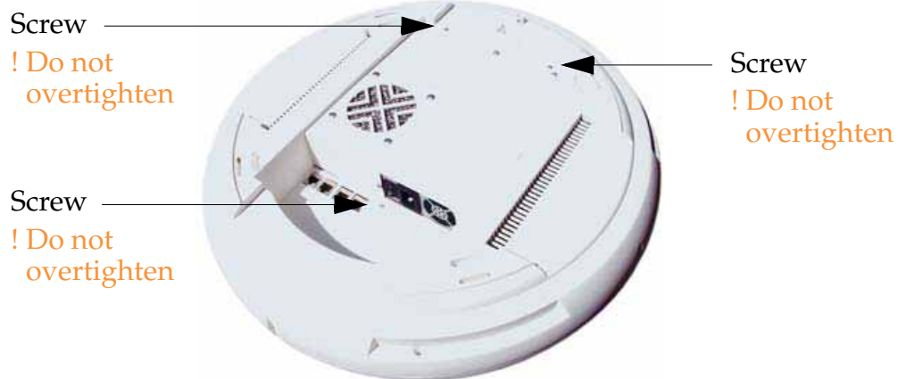
Figure 179. Reinstalling the Access Panel
