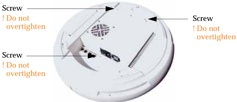
Figure 180. Reinstalling the Access Panel
