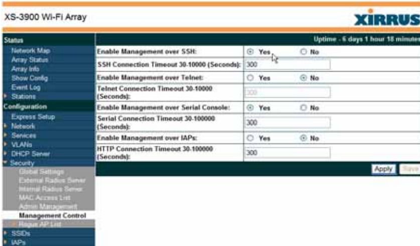
Figure 195. Security/Management Control Window
