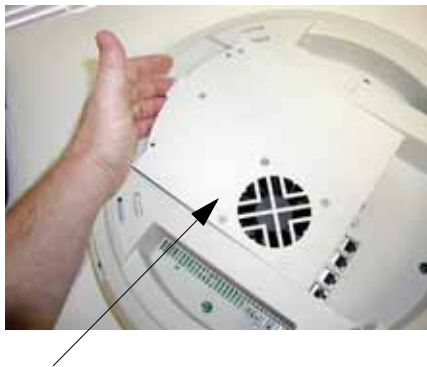
Access panel (with power supply and fan)
