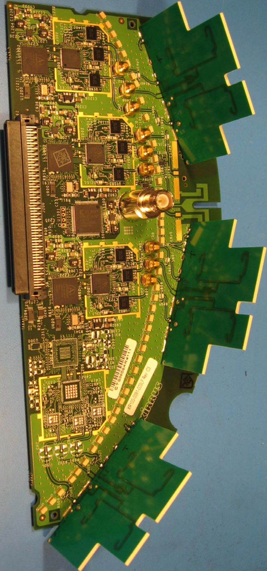
Radio Board (3 Transceivers installed for XN12) Top View
