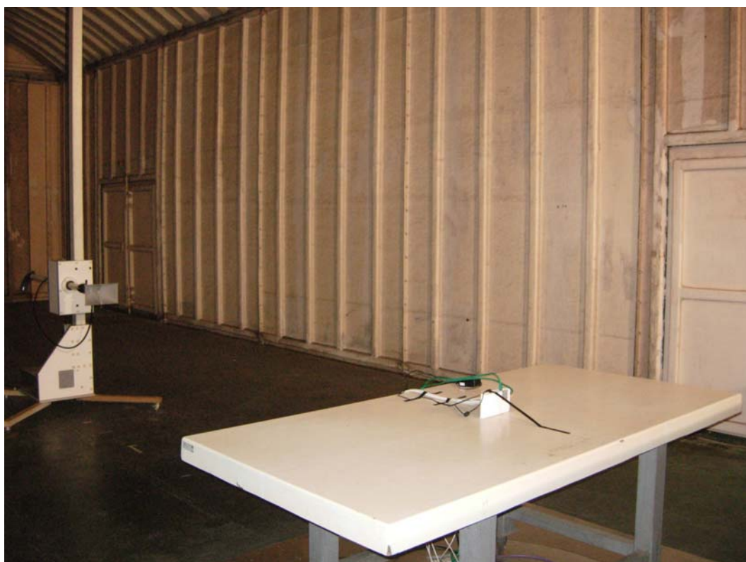
Back View of Radiated Test (Horn)
