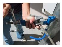
Once the strap is satisfactorily tight, rotate the Band-It tool back so that the strap cannot slide back through the buckle.
