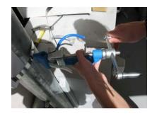
Rotate the Band-It tool so that it can pull the excess strap through the buckle and turn the crank until the strap is very tight.
