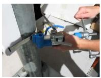
Using the built in cutting tool on the Band-It tool, cut the excess strap.
