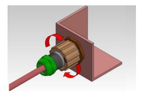
• Snug all the sections of the assembly together a final time and tighten the sealing nut on the end to 5kg but not more than 8kg torque force to insure a water tight fit.
