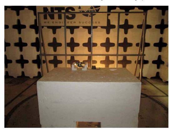
Conducted Emissions Test Configuration Photographs
