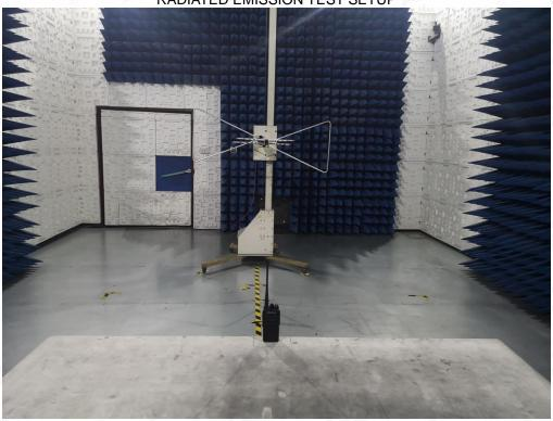
RADIATED EMISSION ABOVE 1G TEST SETUP
