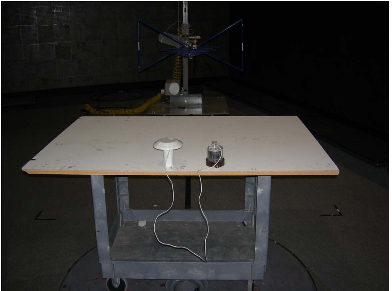
Figure 1: Test Setup Radiated Emissions – Unintentional
