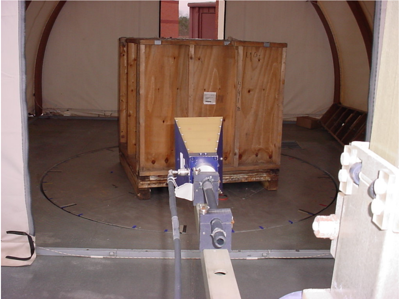
Figure 2: Test Setup Radiated Emissions - Intentional
