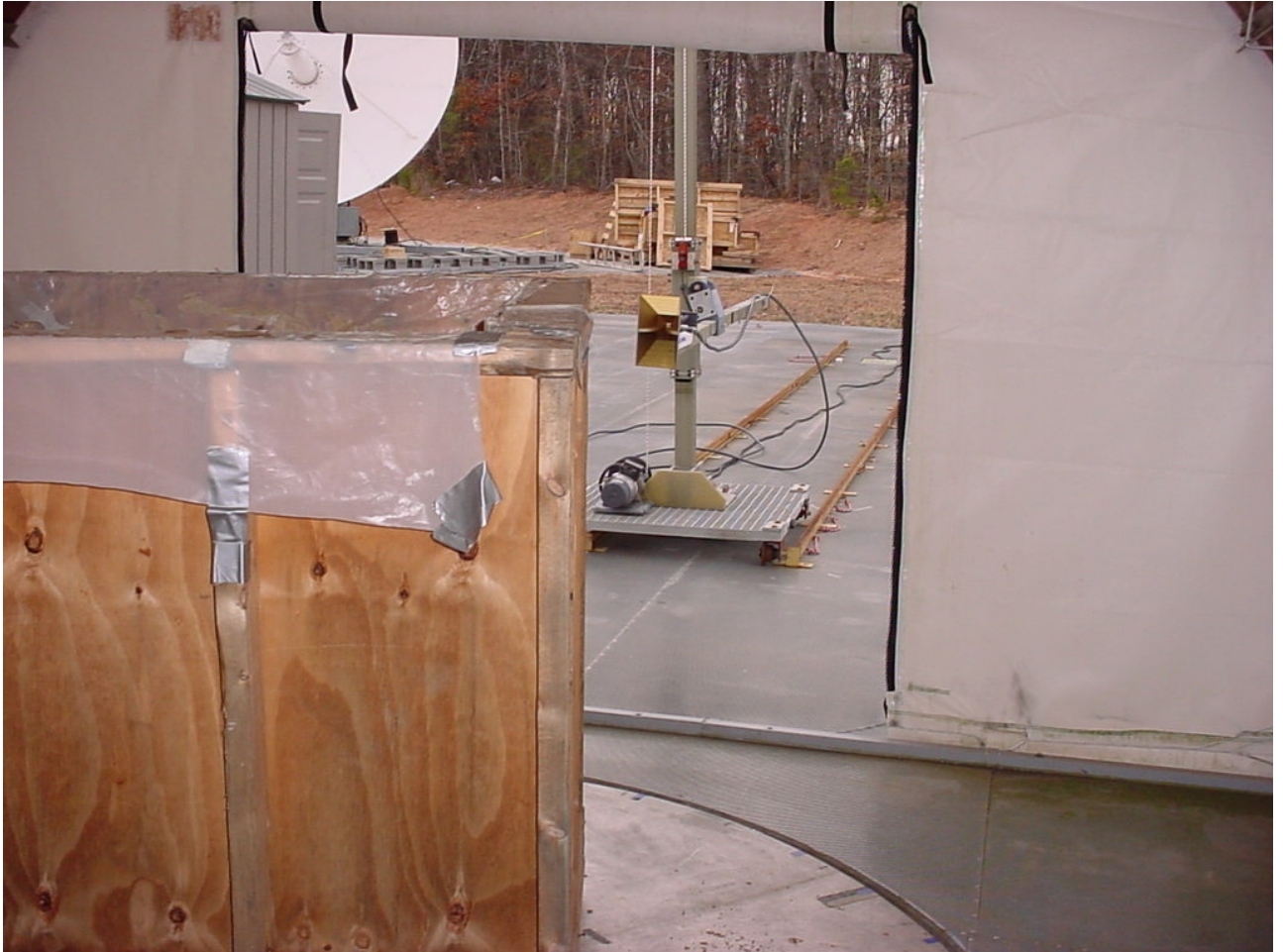
Figure 3: Test Setup Radiated Emissions - Intentional
