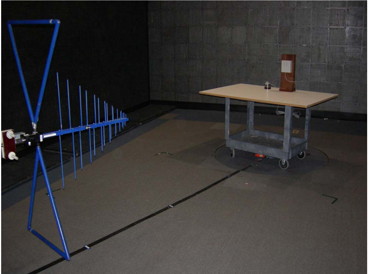
Figure 2: Test Setup Radiated Emissions - Unintentional
