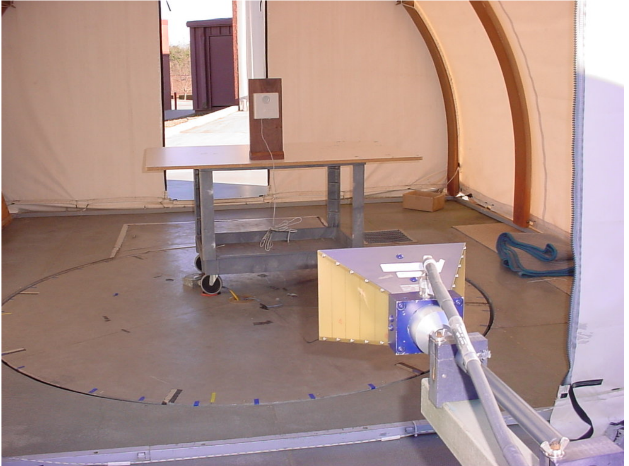
Figure 4: Test Setup Radiated Emissions - Intentional
