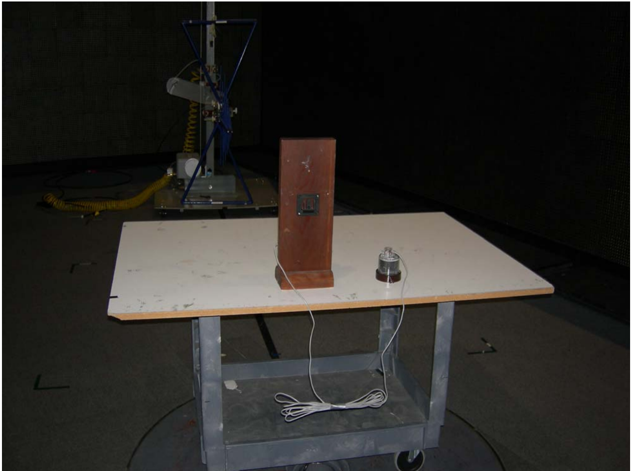
Figure 1: Test Setup Radiated Emissions – Unintentional
