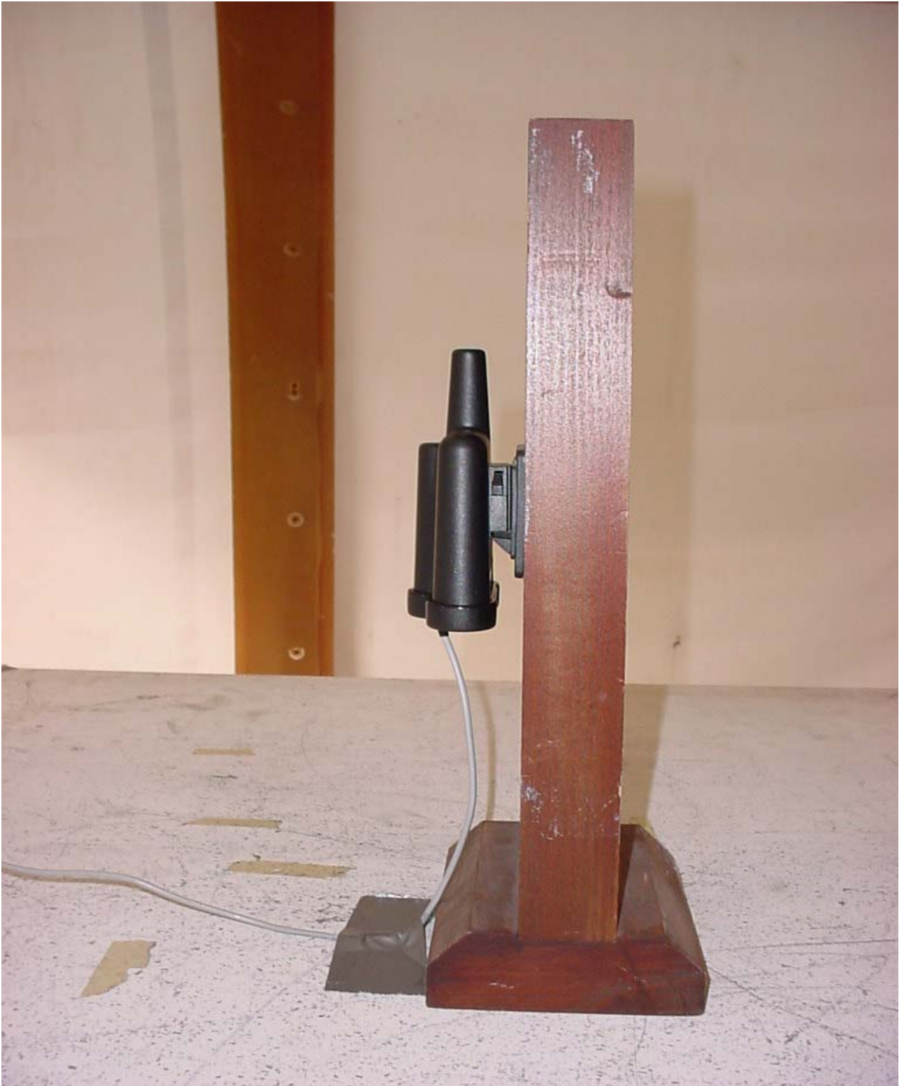
Figure 6: Test Setup Radiated Emissions - Intentional
