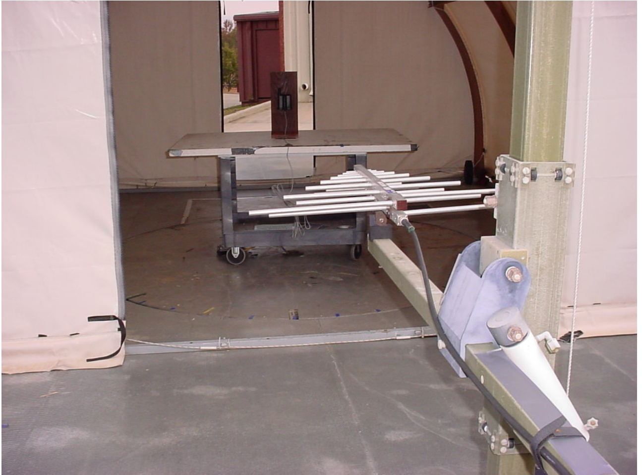
Figure 3: Test Setup Radiated Emissions - Intentional
