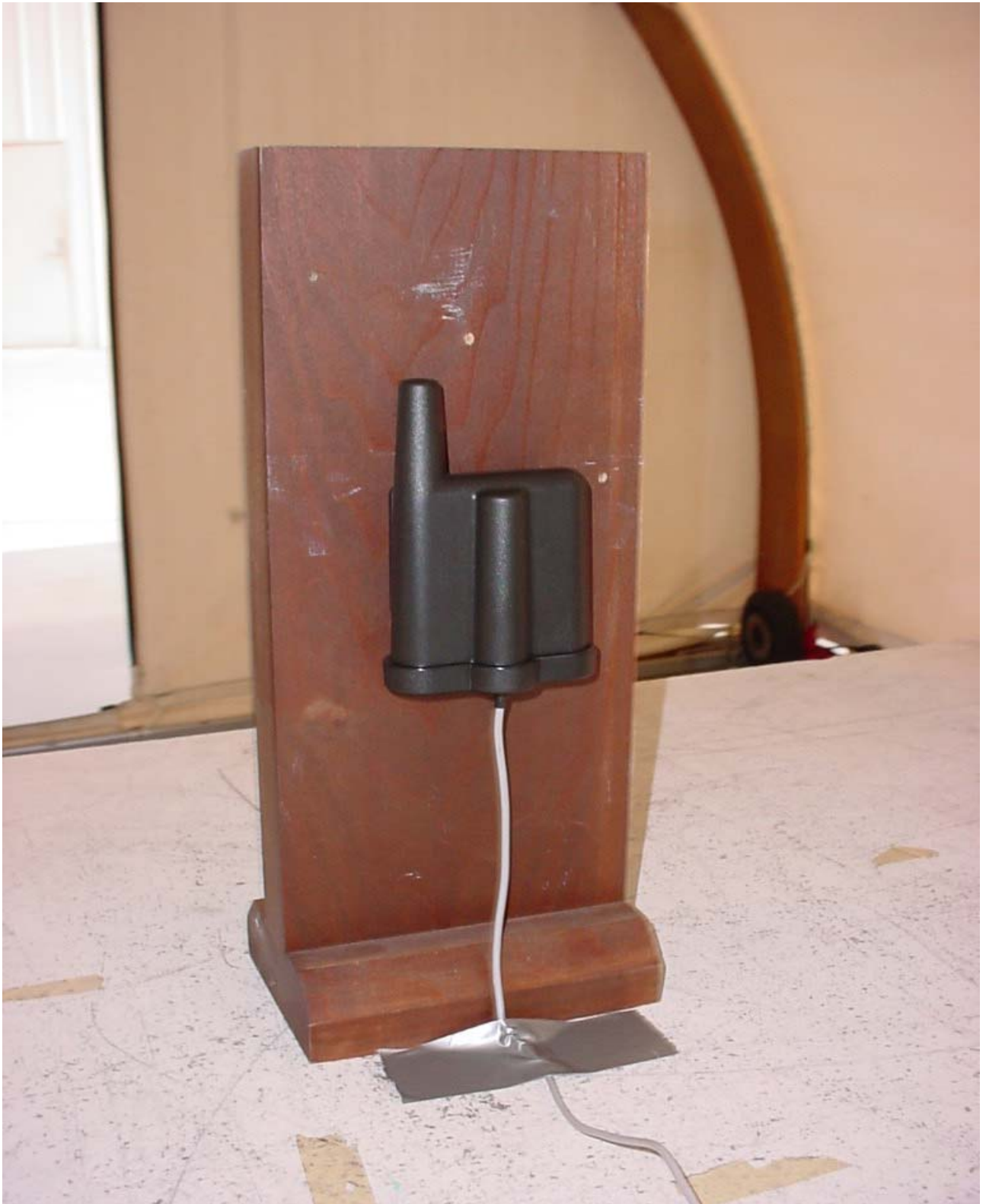
Figure 5: Test Setup Radiated Emissions - Intentional
