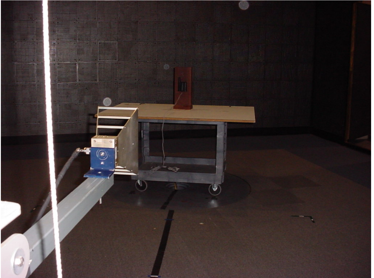
Figure 8: Test Setup Radiated Emissions - Intentional
