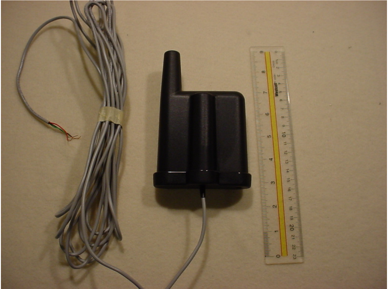
Figure 5: External – Front View with Meter Cable
