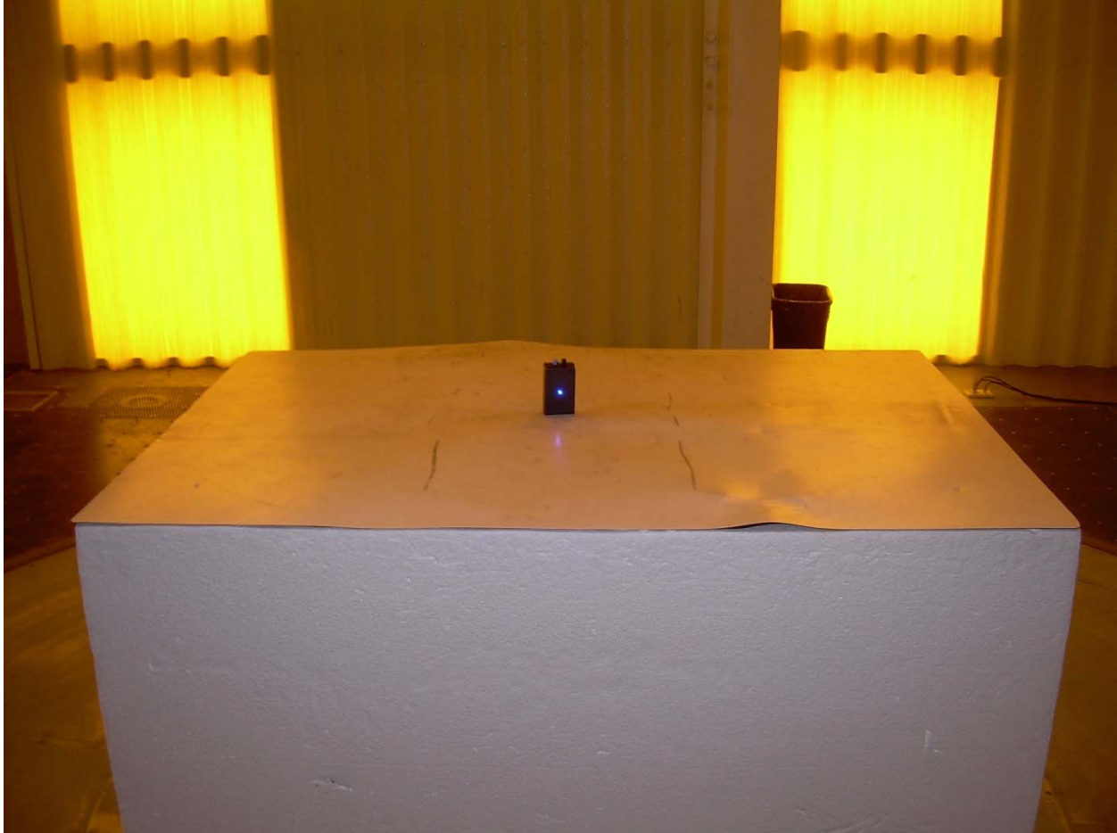
Photograph 1 – Front View Worst-Case Radiated Emissions Setup
