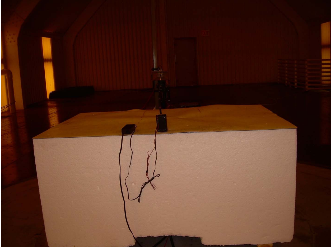
Photograph 2 – Front View Worst-Case Radiated Emissions Setup
