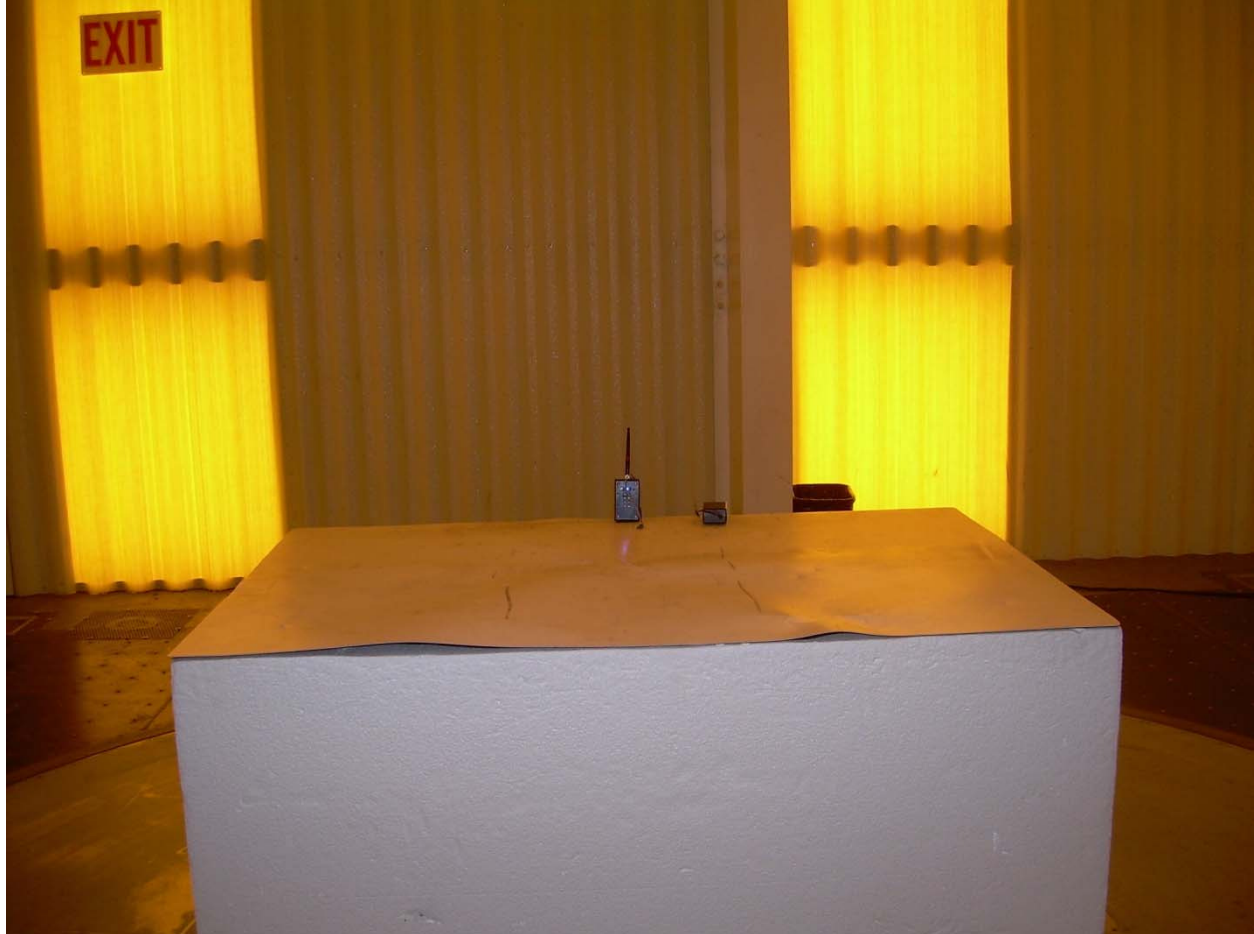
Photograph 1 – Front View Worst-Case Radiated Emissions Setup
