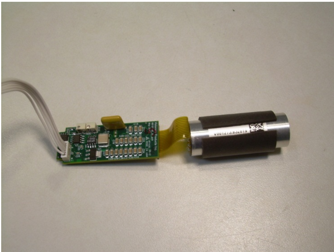
View of the Scintillation Tube and Component Side of the PCB
