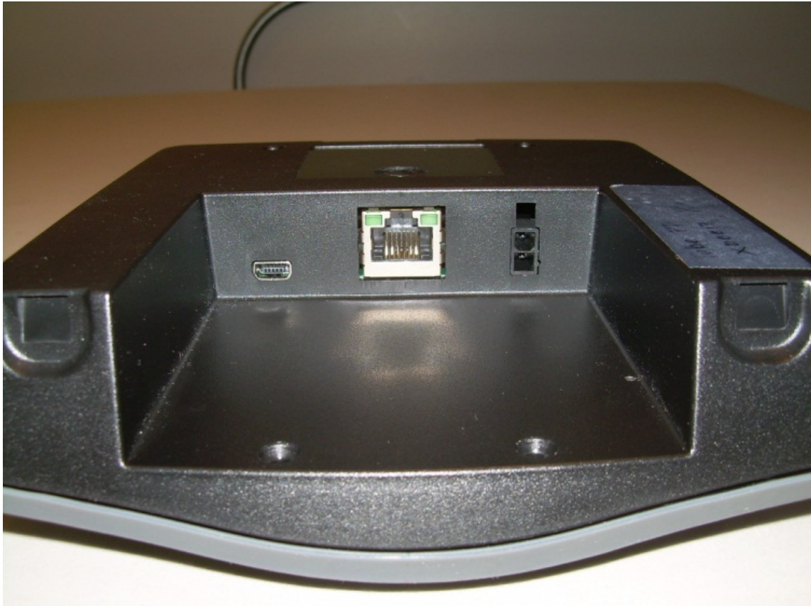
View of the Bottom of the EUT Showing Interface Ports
