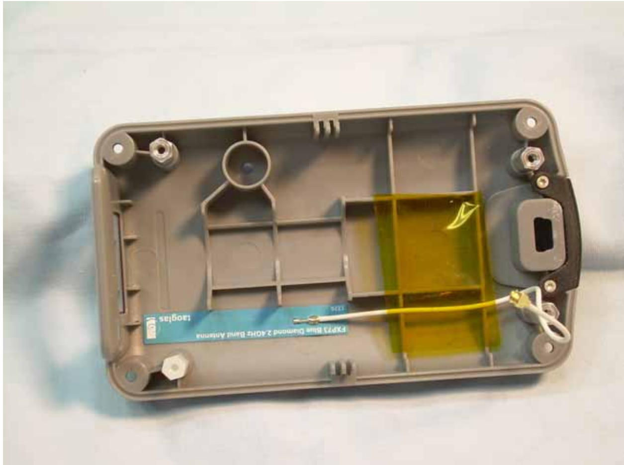
Photograph 18 – View of the 802.15.4 Transceiver Antenna
