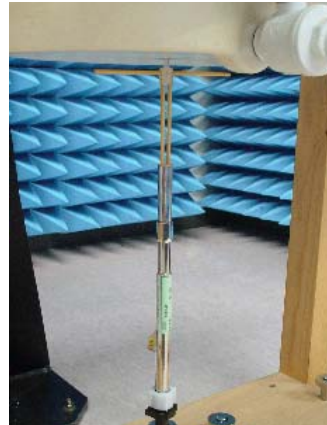
Photograph of the 900MHz dipole Antenna
