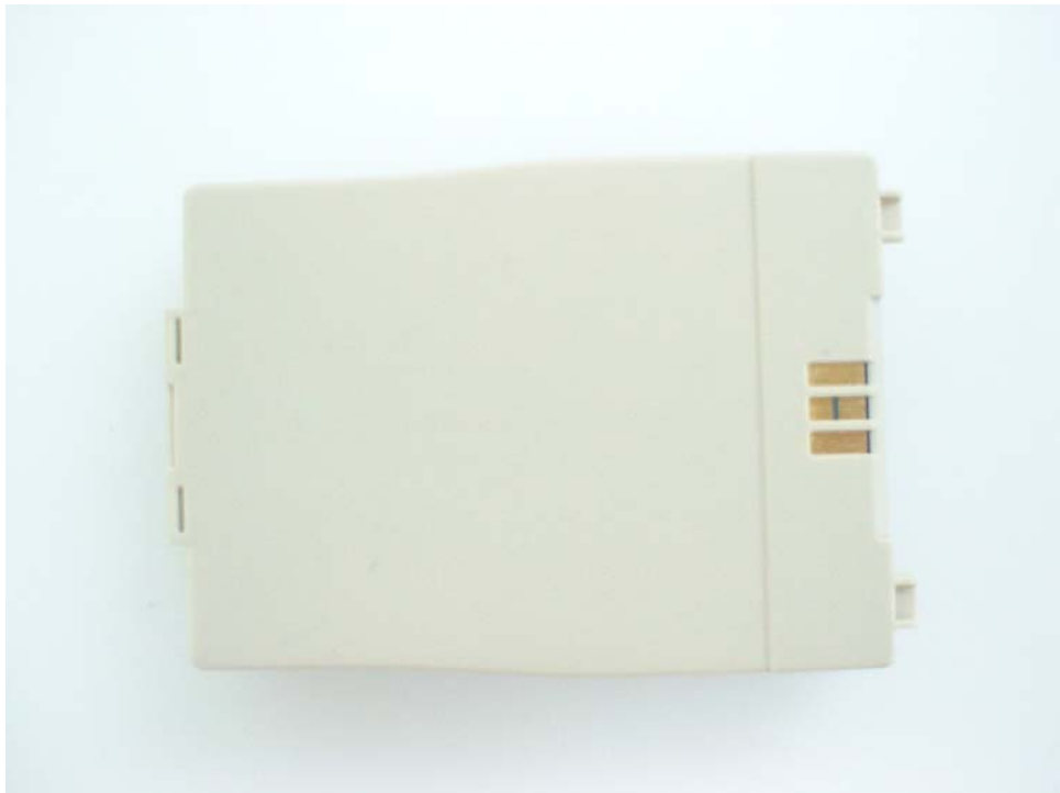
Fig.13 Back view of Battery
