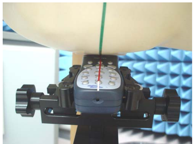
Fig.4 Right Head Section / Cheek-Touch Position
