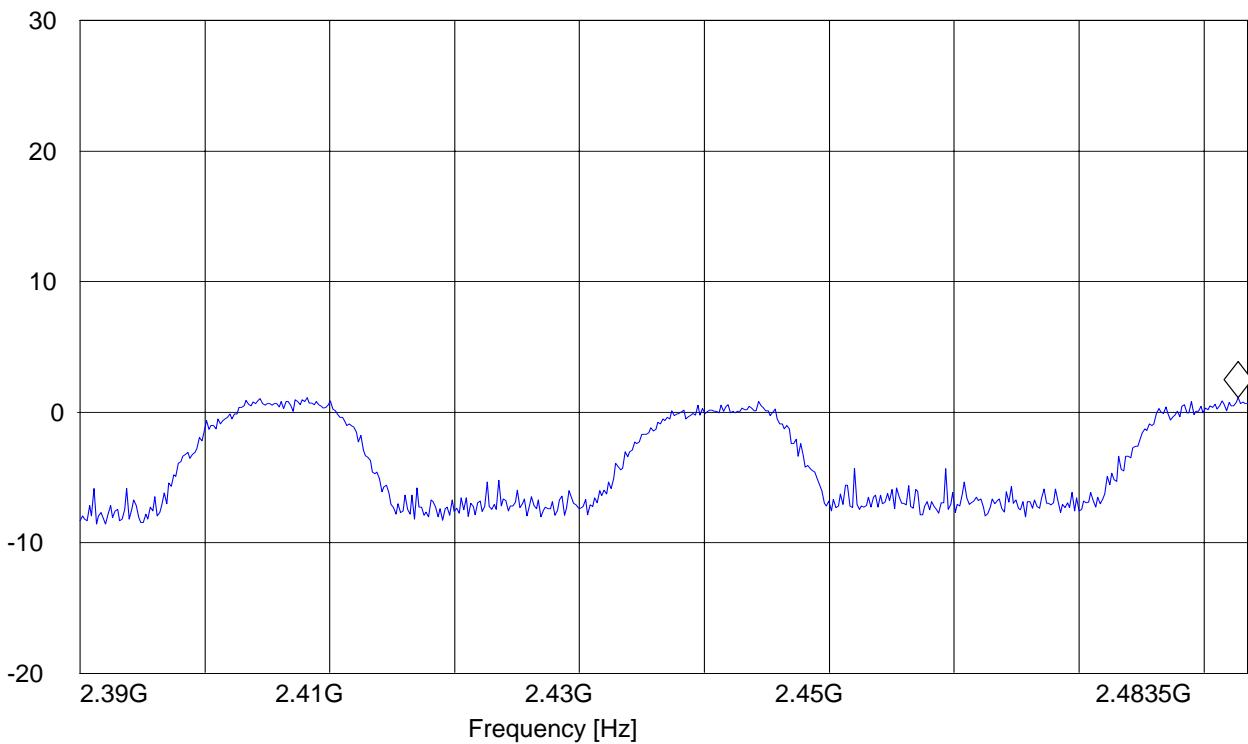
**This plot replaces all the other EIRP measurements only for the high channel (15) due to the fact that it failed banded edges at maximum power. Bandedges were complaint with a lower power setting (7). Being this the case the EIRP for channel 15 at setting of 7 was re-measured as final configuration of the EUT.**
