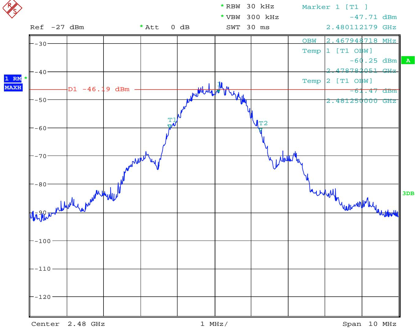
**5.3 POWER SPECTRAL DENSITY §15.247(e) & RSS-210 (A8.2)(b)****(CONDUCTED)****Limit: ≤ 8dBm (in 3kHz BW) §15.247(e) & RSS-210 (A8.2)(b)****ANALYZER SETTINGS: RBW= 3kHz, VBW: 10kHz SPAN: 300kHz**
