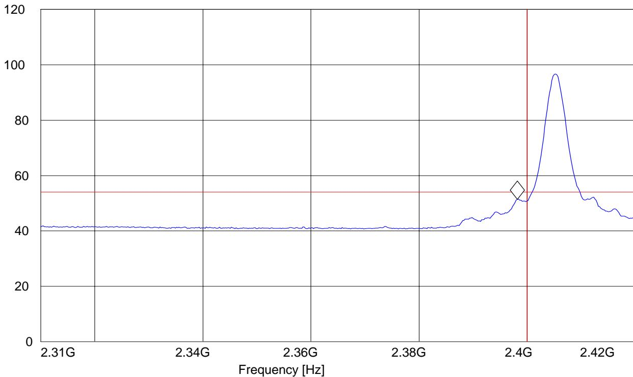
**BAND EDGE COMPLIANCE****§15.247 (d) & RSS-210(A8.5)****High frequency section (spurious in the restricted band 2483.5 – 2500 MHz)**
