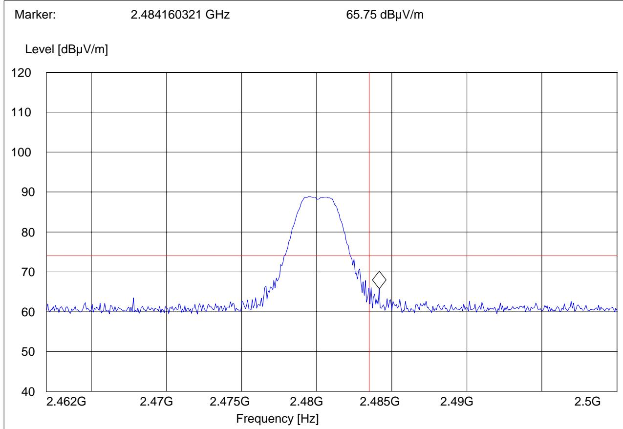
**BAND EDGE COMPLIANCE****§15.247 (d) & RSS-210(A8.5)****High frequency section (spurious in the restricted band 2483.5 – 2500 MHz)**
