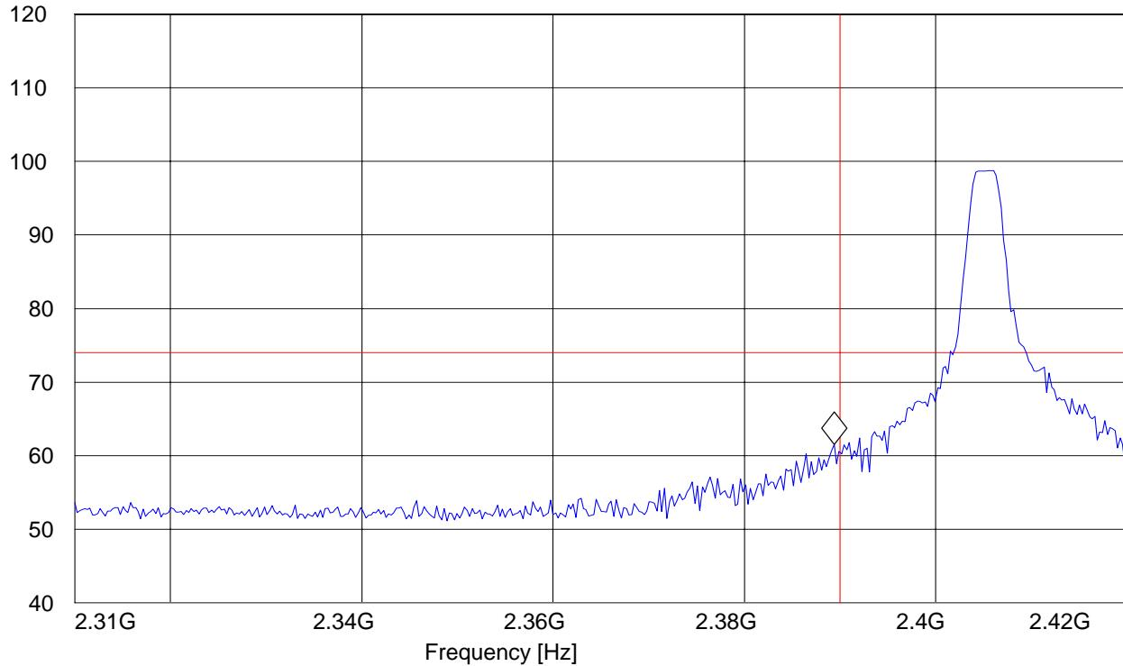
**BAND EDGE COMPLIANCE****§15.247 (d) & RSS-210(A8.5)****Low frequency section (spurious in the restricted band 2310 – 2390 MHz)**
