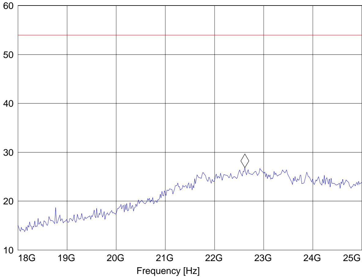
**5.7 EMISSION LIMITATIONS – Radiated (Receiver)****RSS-GEN (4.10) & (6):****Limits RSS-GEN (4.10) & (6):**
