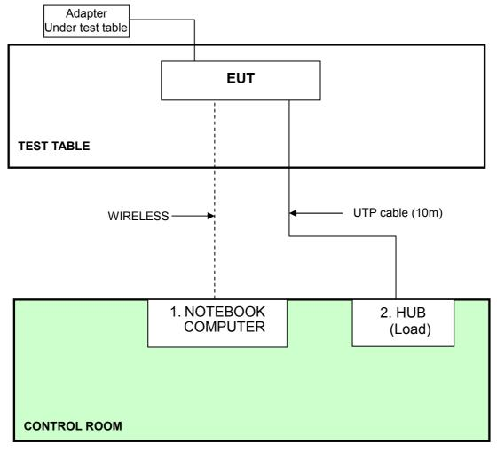
**NOTE:** 1. Support units 1-2 were kept in the control room during the test.
