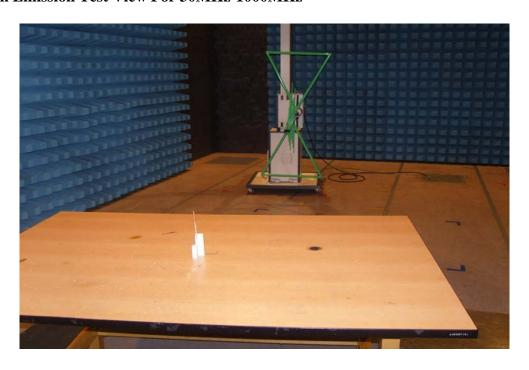
**Radiation Emission Test View For 1GHz-5GHz**
