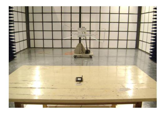
**Radiation Emission Test View For 1GHz-10GHz**
