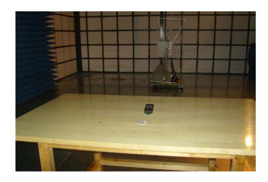
**Radiation Emission Test View For 1GHz-5GHz**
