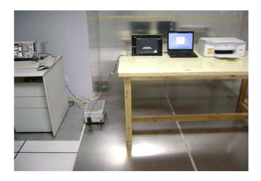
**Radiated Emissions Test Setup**
