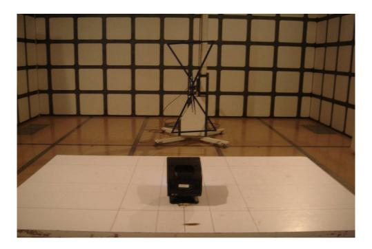
Radiated Emissions Test Setup For 1GHz-5GHz
