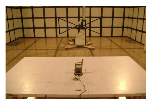
Radiated Emissions Test Setup For 1GHz-5GHz
